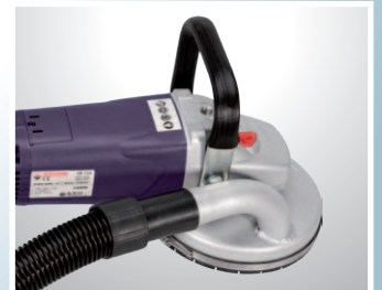
Metal guard with rubber dust-seal and dust-extraction port to industrial vacuum-cleaner, ensuring dustless operation
